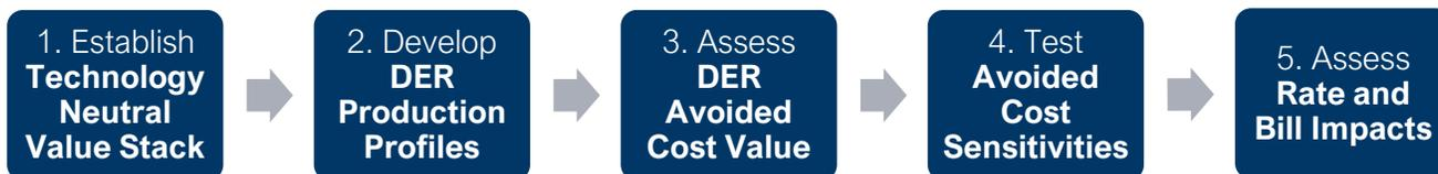
First, baseline technology-neutral avoided cost values are established (step 1). Next, DER production curves are developed for each resource type (step 2) and mapped against the technology-neutral avoided costs to calculate the avoided cost value of DERs by system type (step 3). Avoided cost values are also calculated under sensitivity cases, including consideration of environmental externalities, high
