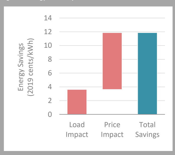
Figure 5. Energy benefits per kWh of BTM solar
