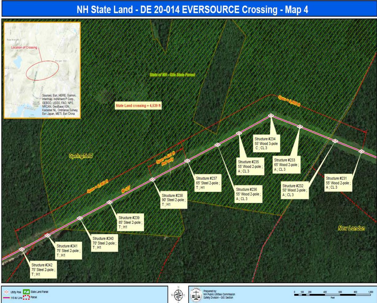
**Figure 1:** 115kV line, designated as the M127 Transmission Line, is a span of approximately 4867 feet between structures # 231 and # 242, crossing approximately 4539 ft. of State land in the Towns of Springfield and Franklin, NH. State owned land is shown above as green hash marks
