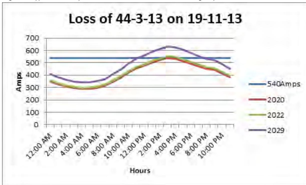
Figure 6: Typical Peak Day Load Profiles for Circuit 44-3-13 Contingency on Circuit 19-11-13
