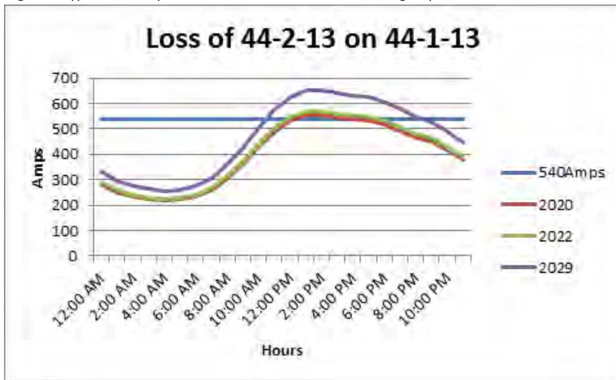
Figure 4: Typical Peak Day Load Profiles for Circuit 44-2-13 Contingency on Circuit 44-1-13
