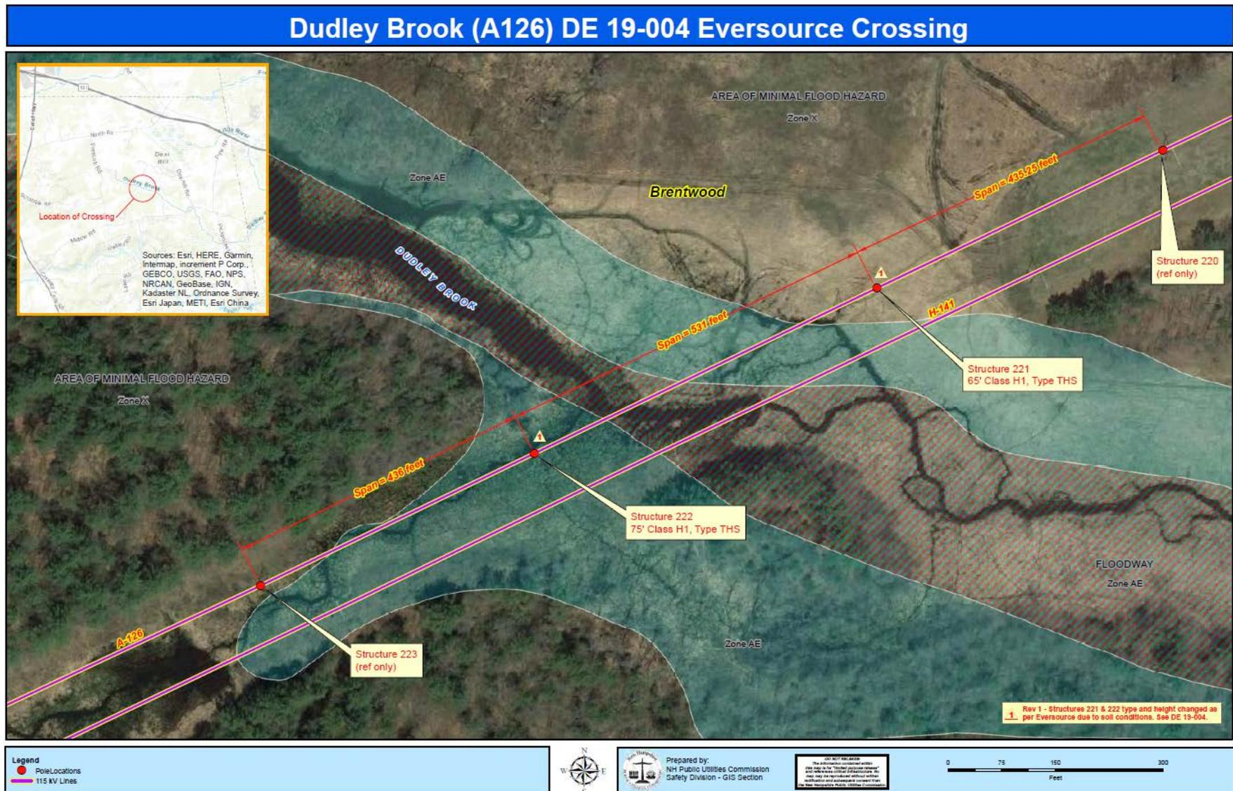
**Figure 1:** 115kV line, designated as the A126 Transmission Line, is a span of approximately 531 feet between structures #221 and # 222, across the Dudley Brook in Brentwood, NH.
