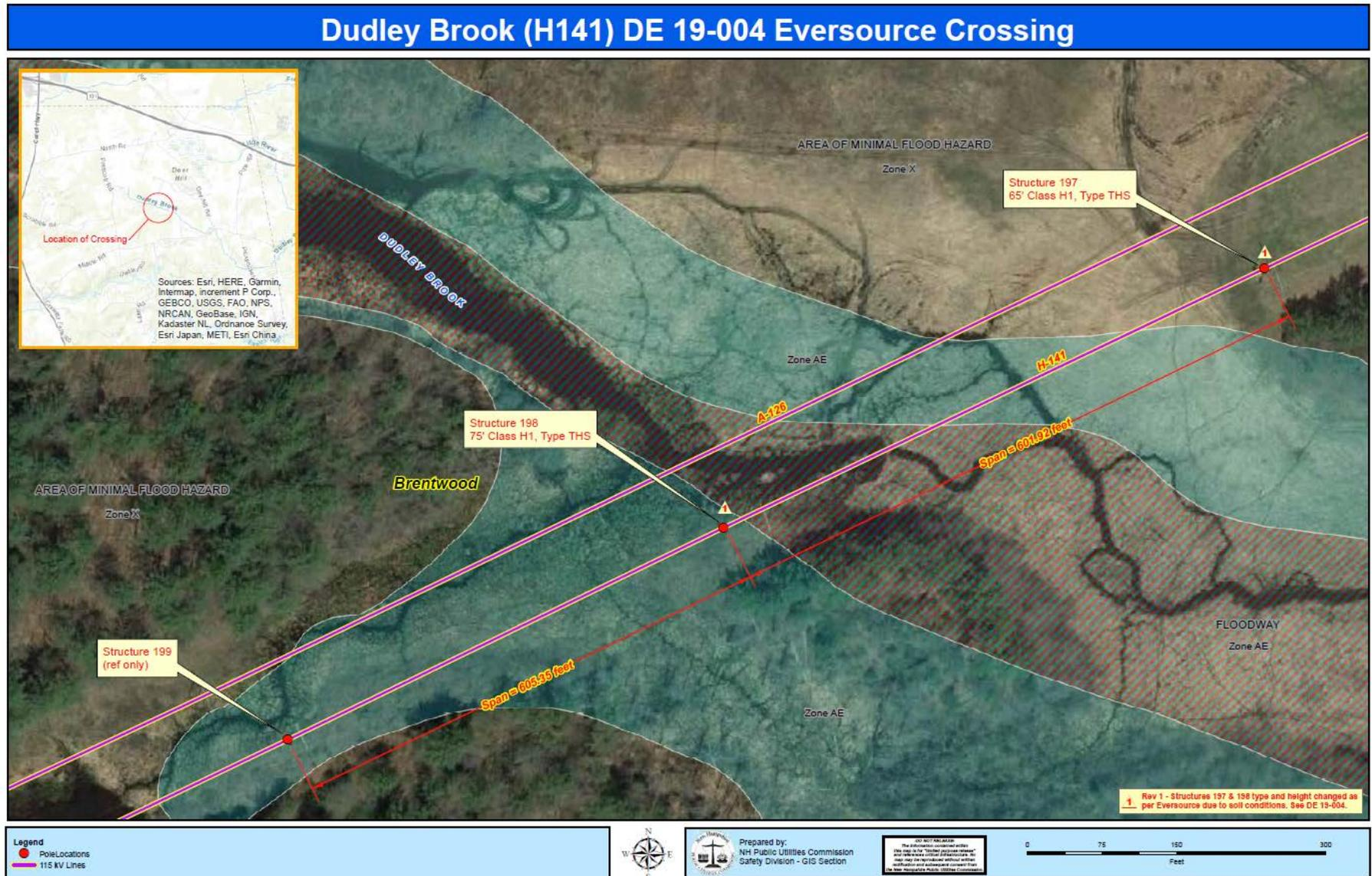
**Figure 1:** 115kV line, designated as the H141 Transmission Line, is a span of approximately 601.92 feet between structures # 197 and #198, across the Dudley Brook in Brentwood, NH.
