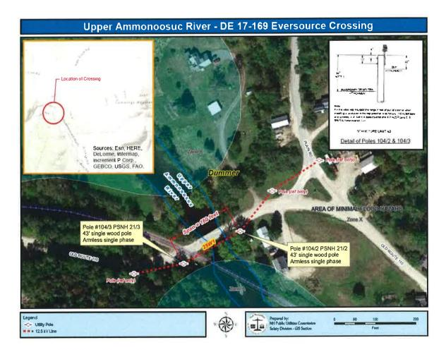
**Figure 1:** 7.2 kV, designated as the 25W1 Circuit, a span of approximately 160 feet, across the Upper Ammonoosuc River in Dummer, NH. The structures on the south side of the bridge are armless structures designated #21/3 and #21/2 to be constructed with a single class-2, 50 foot tall, CCA pole (embedded 7 feet). The span of the river is approximately 100 feet at the east and west banks, with the span from pole to pole 160 feet.
