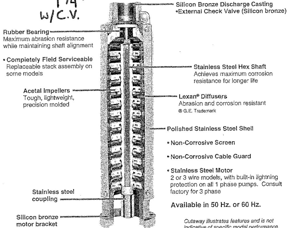
*Cutaway illustrates features and is not indicative of specific model performance.*
