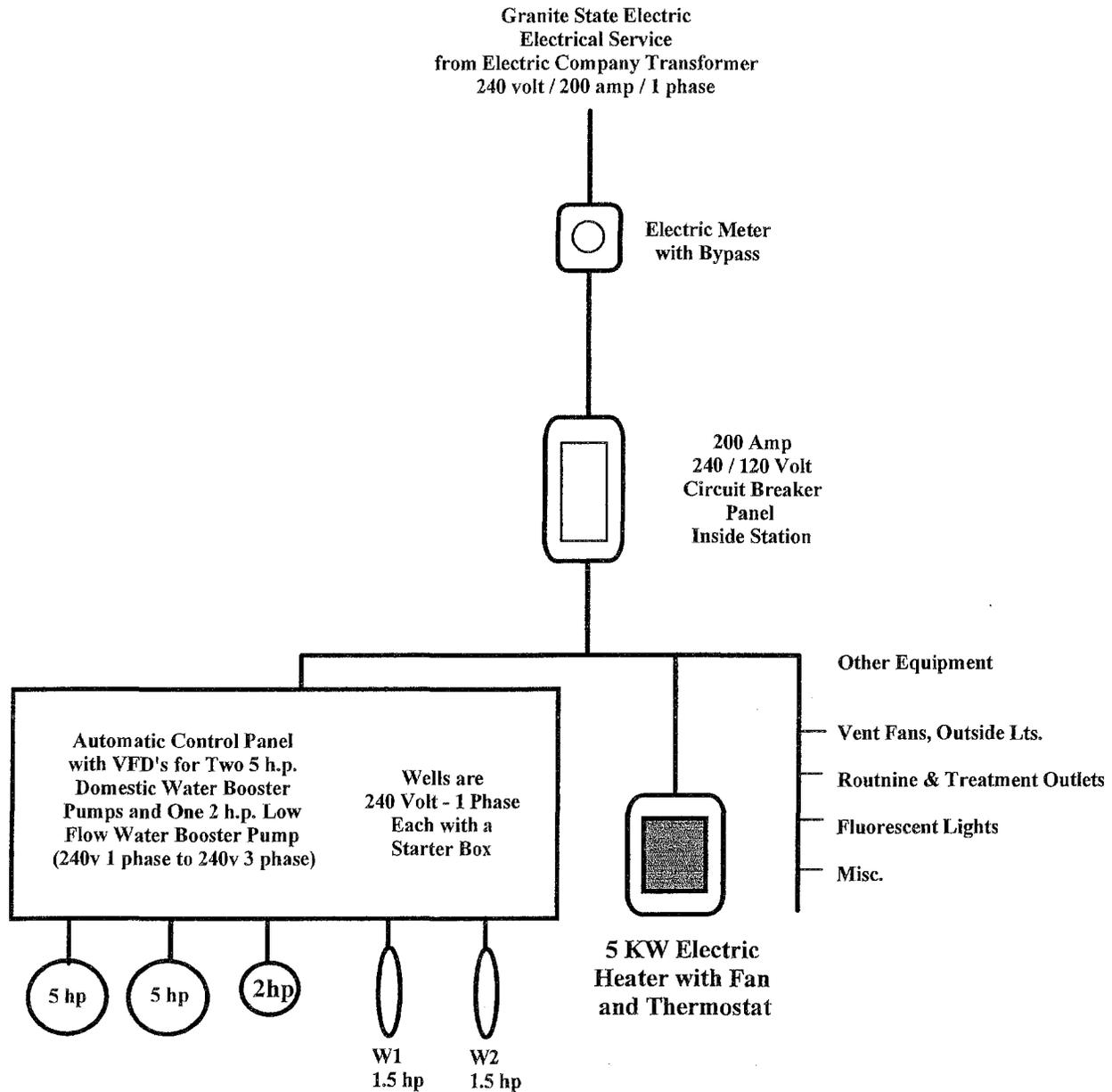
**Note:** All wiring to meet National and Local Electrical Code. All wire to be run in PVC or EMT conduit. Liquid tight allowed between motors and conduit. All enclosures minimum NEMA I Fluorescent lighting to each be 4' as needed, twin tube, moisture resistant.
