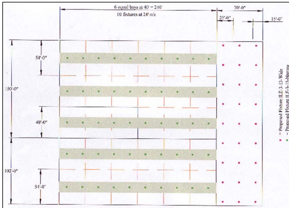
Figure 4-2 Proposed Cooler Lighting Configuration
