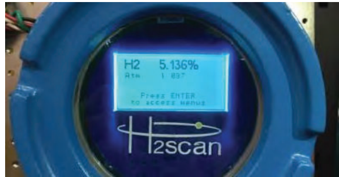
Figure 5.4 H2Scan's HY-OPTIMA 2700 Series analyzer outputs hydrogen concentration in real time
