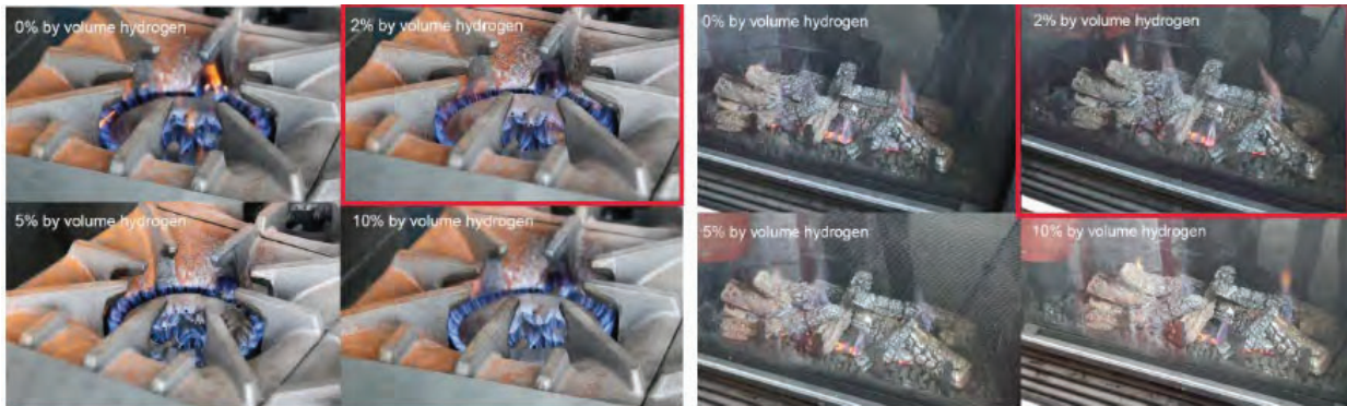
Figure 5.3 Stove (left) and fireplace (right) images of natural gas-hydrogen blends from 0% to 10% hydrogen by volume, sourced from Enbridge [6]
