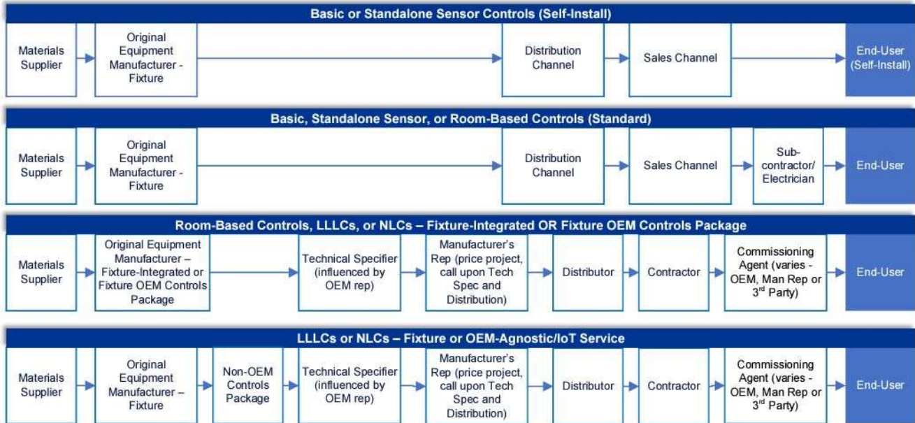
Figure 5-18. Simplified supply chain mapping for control categories 205
