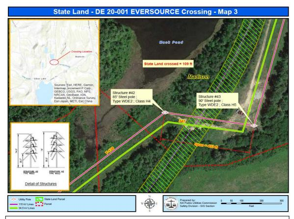
**Figure 3:** 115kV line, designated as the Y138 Transmission Line, is a span of approximately 453 feet between structures # 42 and # 43, with a span of approximately 109 ft. crossing State Land in the Town of Madison, NH. State owned land is shown above as green hash marks
