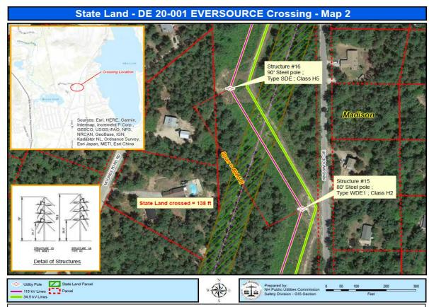
**Figure 2:** 115kV line, designated as the Y138 Transmission Line, is a span of approximately 494.5 feet between structures # 15 and # 16, with a span of approximately 138 ft. crossing State Land in the Town of Madison, NH. State owned land is shown above as green hash marks
