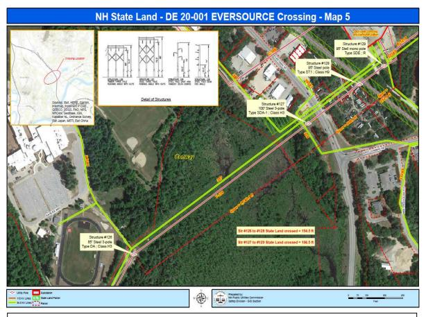
**Figure 4:** 115kV line, designated as the Y138 Transmission Line, is a span of approximately 2499.5 feet between structures # 126 and # 129, with a span of approximately 261 ft. crossing State Land in the Town of Conway, NH. State owned land is shown above as green hash marks
