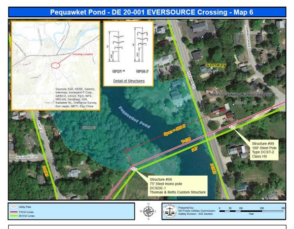
**Figure 4:** 115kV line, designated as the Y138 Transmission Line, is a span of approximately 505 feet between structures # 98 and # 99, with a span of approximately 172 ft. crossing the Pequawket Pond in the Town of Conway, NH. State owned land is shown above as green hash marks
