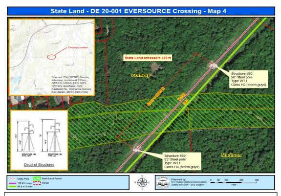
**Figure 4:** 115kV line, designated as the Y138 Transmission Line, is a span of approximately 800.5 feet between structures # 89 and # 90, with a span of approximately 370 ft. crossing State Land in the Town of Conway, NH. State owned land is shown above as green hash marks
