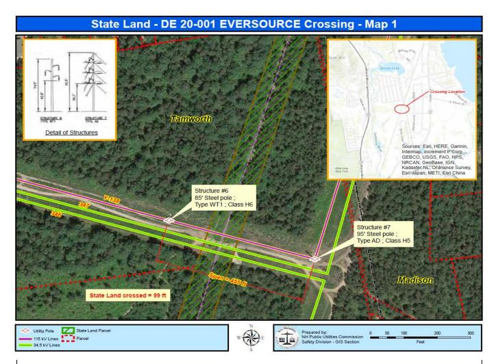
**Figure 1:** 115kV line, designated as the Y138 Transmission Line, is a span of approximately 455 feet between Structure #6 and Structure #7, with a span of approximately 99 ft. crossing State Land in the Town of Tamworth, NH. State owned land is shown above as green hash marks
