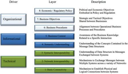
Fig. 3.16 The GridWise Architecture Council interoperability framework [27, 28]
