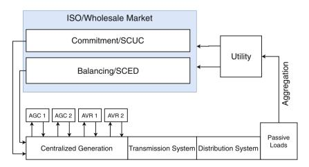
Fig. 3.14 A generic hierarchical control structure for a typical power system area
