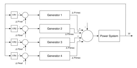
Fig. 3.6 Schematic of automatic generation control [20]
