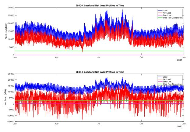
Figure 7: The load and net load profiles from Scenario 2040-4 (top) and 2040-3 (bottom).
