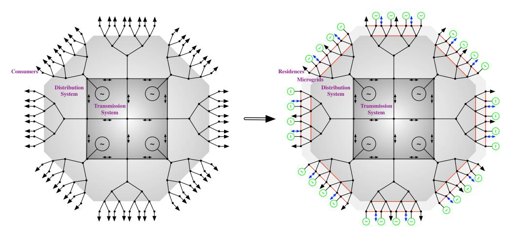
The integration of distributed energy resources at the grid's periphery implies the adoption of a plethora of network-enabled devices and appliances in an energy Internet of Things.
