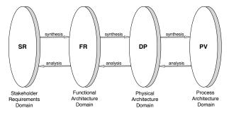
Fig. 1. Four Domains in the Engineering Design of Systems – An Axiomatic Design Perspective (Adapted from [3])
