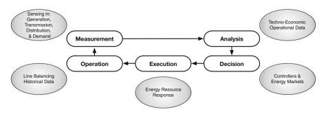
Fig. 1.1 A closed-loop framework for electrical power system management
