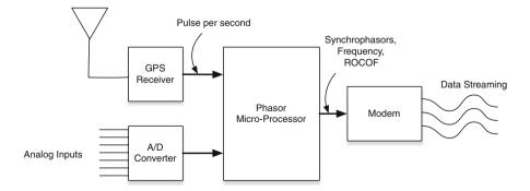
Fig. 3.5 Schematic of a Phasor measurement unit [20]
