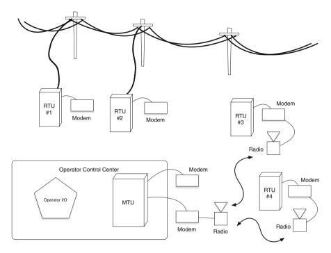
Fig. 3.4 SCADA as a network of remote terminal units (RTUs) connected to a master terminal unit (MTU) via modems and radios [19]
