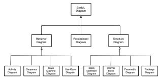
Fig. 3. Taxonomy of SysML Diagrams (Adapted From [18], [19])
