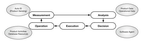
Fig. 1.8 A closed-loop control framework for production systems with intelligent products [5-13]
