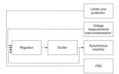
Fig. 3.7 Schematic of automatic voltage regulation [20]
