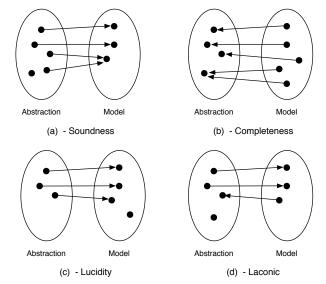
Fig. 11. Graph Theoretical Representation of Mapping between a Model and its Abstraction: (a) Soundness (b) Completeness (c) Lucidity (d) Laconicity [64].
