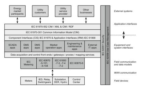
Fig. 3.18 An overview of important eIoT standards (adapted from [29])
