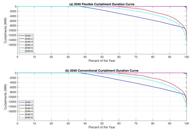
Figure 11: Curtailment duration curves for all six 2040 scenarios in both the flexible (above) and conventional (below) operating modes.
