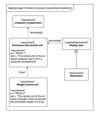
Fig. 5. An Example Requirements Diagram in SysML
