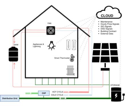
Fig. 4.4 An example eIoT-enabled smart home: DERs are connected to the grid through a cloudbased framework (adapted from [30])
