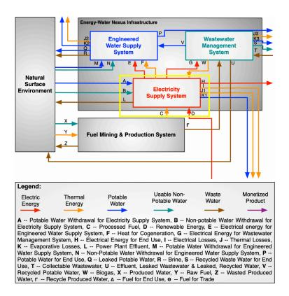
Figure 3: A diagram of the physical flows between the physical infrastructures (water supply system, wastewater management system, and electricity supply system) and the natural surface environment. [49]
