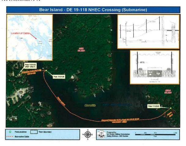
**Figure 1: (2)** Single-phase 7,200 kV Distribution Submarine Cables a span of approximately 4100 feet, under Lake Winnipesaukee from Pine Island to Bear Island in Meredith, NH, at the east and west banks. The structure on the west side of the lake crossing is NHEC Pole #11511/6 on Pine Island and the structure on the east side of the lake crossing, is NHEC Pole #11525/1 on Bear Island. The span of the lake crossing from pole to pole is approximately 4100 Ft.
