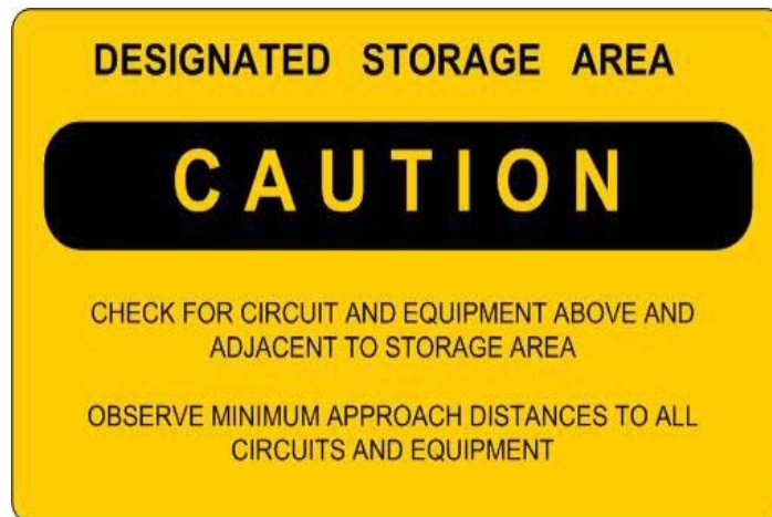
Figure 9 - Substation Designated Storage Area Sign
