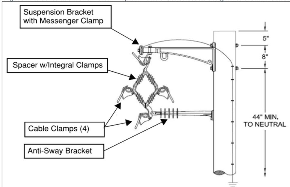
Figure 5-7 above from Standard DTR 10-738 illustrates a 35 kV three phase spacer cable tangent pole and components. The three 35 kV cables are clamped into their positions on the spacer and the spacer is suspended from the messenger wire. The messenger is then installed and secured to the metal suspension bracket. The anti-sway bracket is used to restrict the movement of the spacer cable assembly and is not used on every pole.
