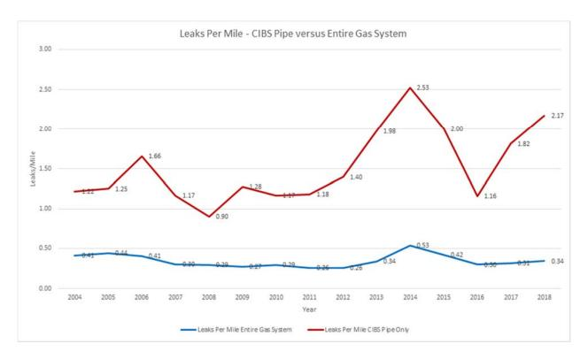
The leaks per mile of on the remaining CIBS pipe is actually higher now than it was when the CIBS program started ten years ago. Even though the Company has removed half of the CIBS pipe, the system experienced a similar number of CIBS breaks in 2018 (six) as during the early years of the program (two in 2005, five in 2006, and six in 2007):
