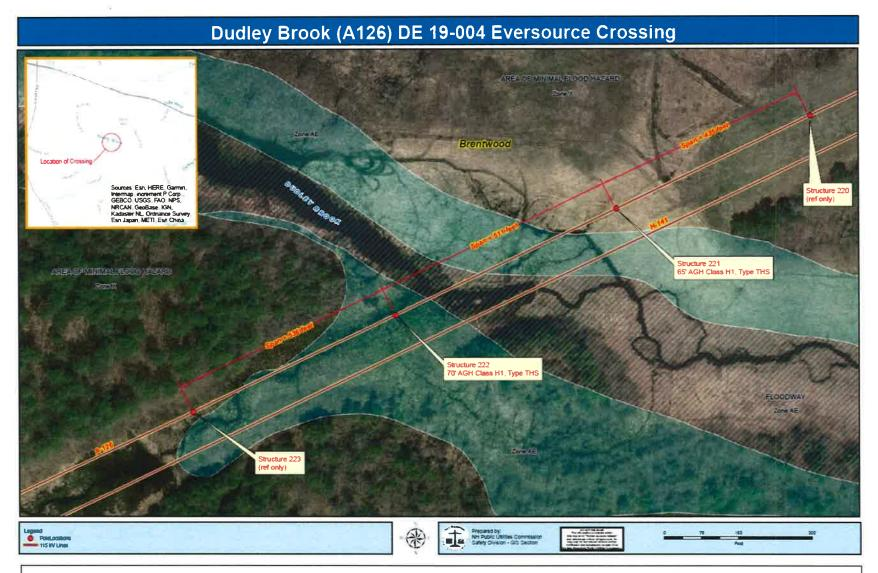
**Figure 1:** 115kV line, designated as the A126 Transmission Line, is a span of approximately 511 feet between structures #221 and # 222, across the Dudley Brook in Brentwood, NH.
