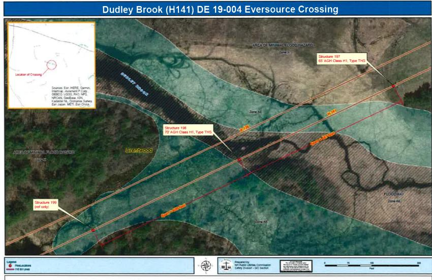
**Figure 1:** 115kV line, designated as the H141 Transmission Line, is a span of approximately 586.92 feet between structures # 197 and #198, across the Dudley Brook in Brentwood, NH.
