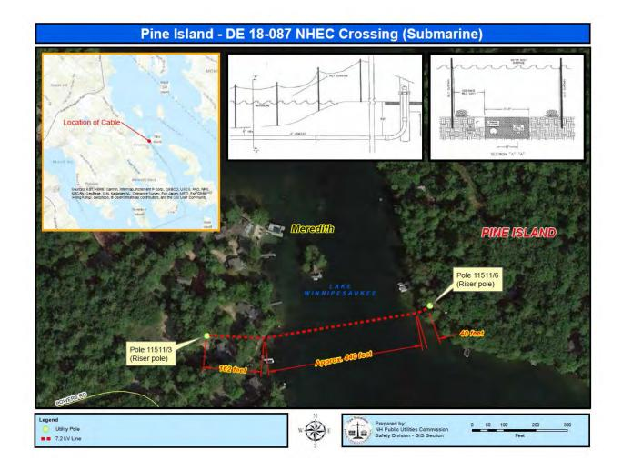
**Figure 1:** (2) Single-phase 7,200 kV Distribution Submarine Cables a span of approximately 440 feet, under Lake Winnipesaukee to Pine Island in Meredith, NH, at the east and west banks. The structure on the west side of the lake crossing is NHEC Pole #11511/3 and the structure on the east side of the lake crossing, is NHEC Pole #11511/6. The span of the lake crossing from pole to pole is approximately 612 Ft.
