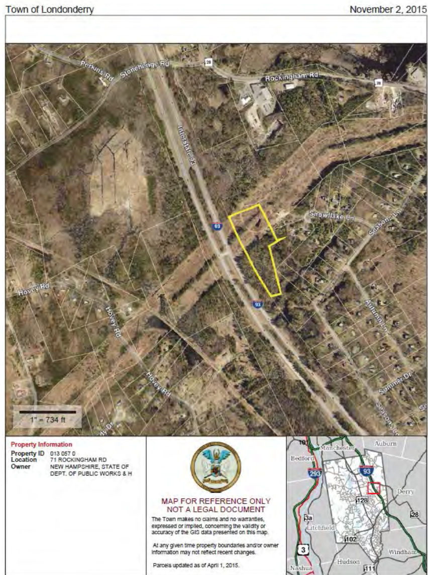
Figure 2: 345kV, designated as the 3124 Line, a span of approximately 548 feet and another of 458 ft, Londonderry, NH. The yellow highlighted parcel is the public land owned by NH DOT that the petition seeks to cross. This is outside of the Highway ROW thus RSA 231:161 does not apply. RSA 371:17 is applicable. The structure on the east side of the Interstate 93 at mile marker 13.8 is new structure 278 and will be located within the Parcel. Structure 278 is a 115 ft tall steel tubular 2 pole H Frame tangential structure with horizontal spacing of the conductors. Structure 279 is identical to Structure 278 except it is located on PSNH property. Note this crossing is referenced as Crossing #2 in this Staff Memorandum and consists of one partial span and one full span is for approximately 21 feet and 451 feet respectively.
