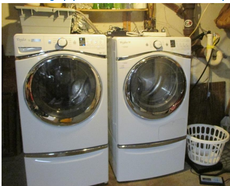
Figure 2. Metering Equipment with New Washer and Heat Pump Dryer
