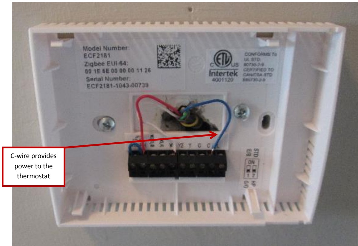
Figure 24. EcoFactor Thermostat with C-wire
