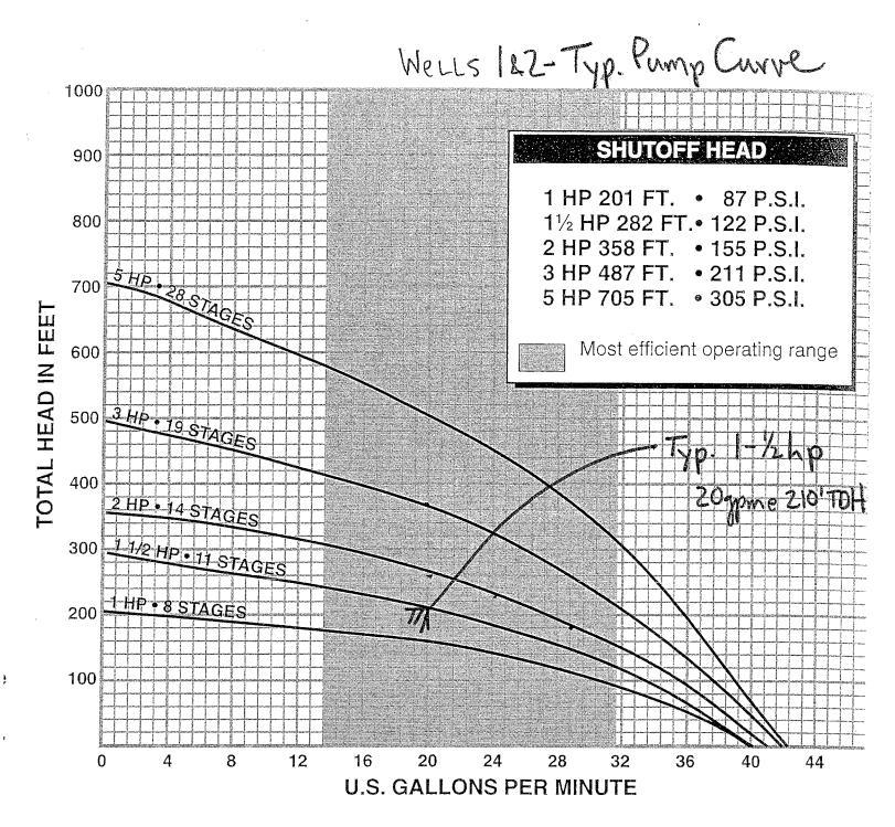
se motors, including 200 volt (575V 1 1/2 HP and larger). ligits of model number. Example: 21100M
