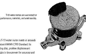
Every T-10 water meter meets or exceeds the latest AWWA C700 Standard. Its nutating disc, positive displacement principle is time-proven for accuracy and dependability since 1892, ensuring maximum utility revenue.
