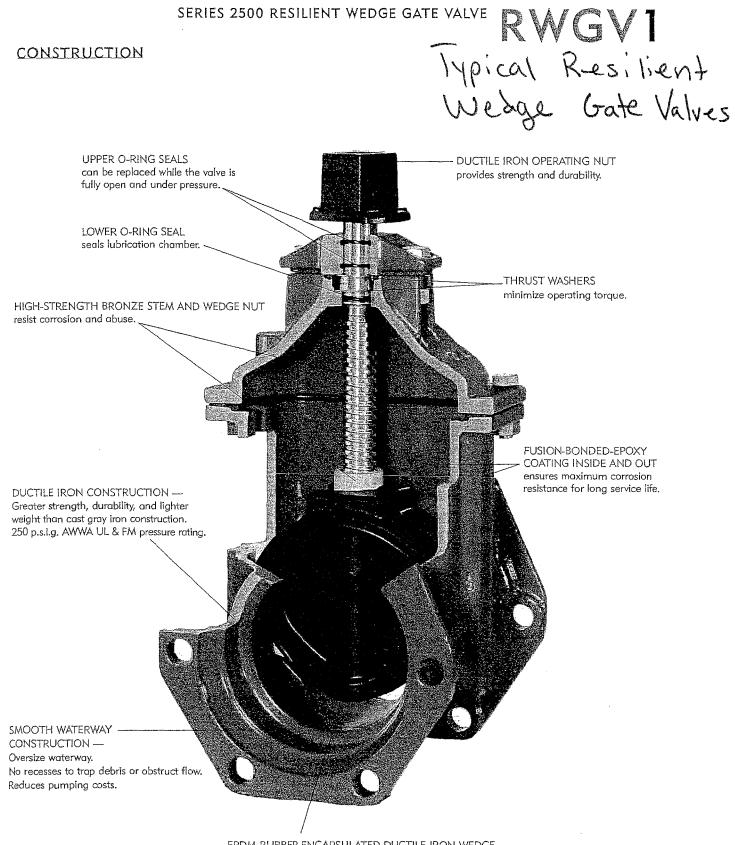
EPDM RUBBER-ENCAPSULATED DUCTILE IRON WEDGE ensures drop tight seal every time with low stem torque.
