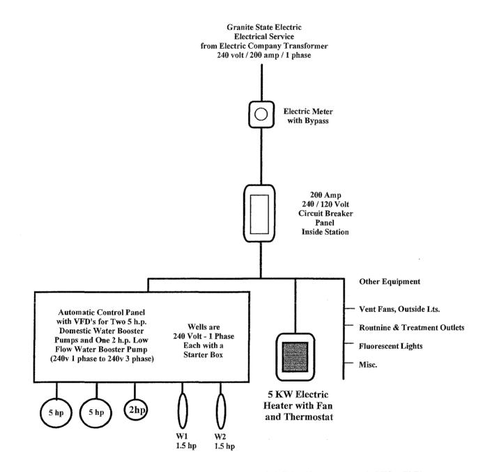
Note: All wiring to meet National and Local Electrical Code. All wire to be run in PVC or EMT conduit. Liquid tight allowed between motors and conduit. All enclosures minimum NEMA I Fluorescent lighting to each be 4' as needed, twin tube, moisture resistant.
